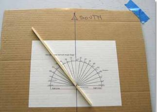
Elevation and azimuth gages in use.
